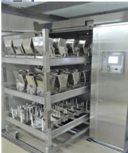
Rack with critical process equipment being loaded into Equipment Washer Disinfector for COP
