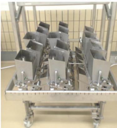
The racks are designed according to the customer’s needs, which ensure an optimal and efficient coverage with the cleaning fluid with a sufficient flow. This contributes to a complete coverage of the surfaces, so that the optimal mechanical washing effect is reached on the specific process equipment. Thus, ensures a more efficient washing process.
